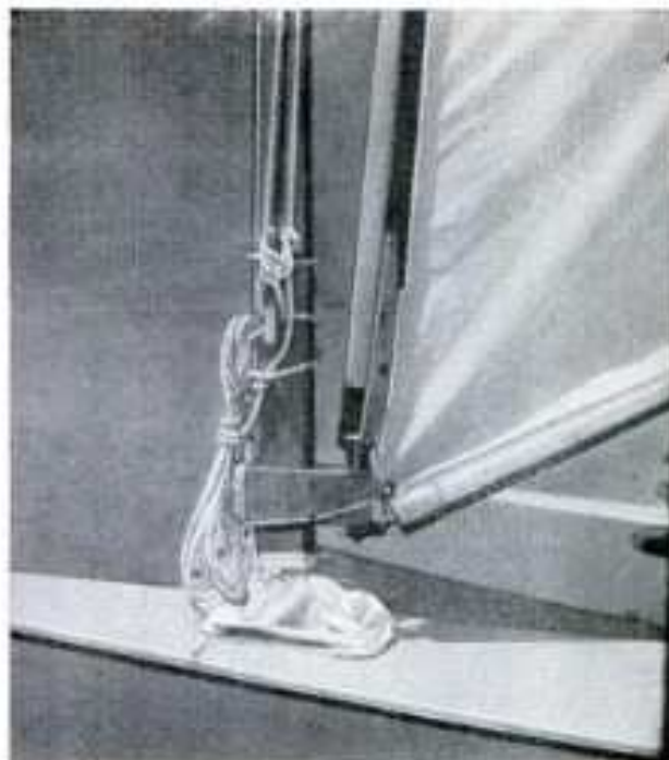
Gooseneck fastened to mast has fittings for attaching boom and lower end of gaff for lateen-type sail
