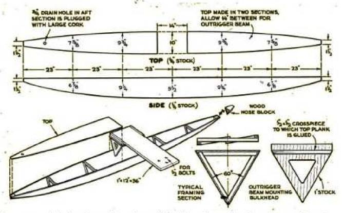
Pontoons are bolted to the outrigger beam. This allows dismantling boat into smaller units.
