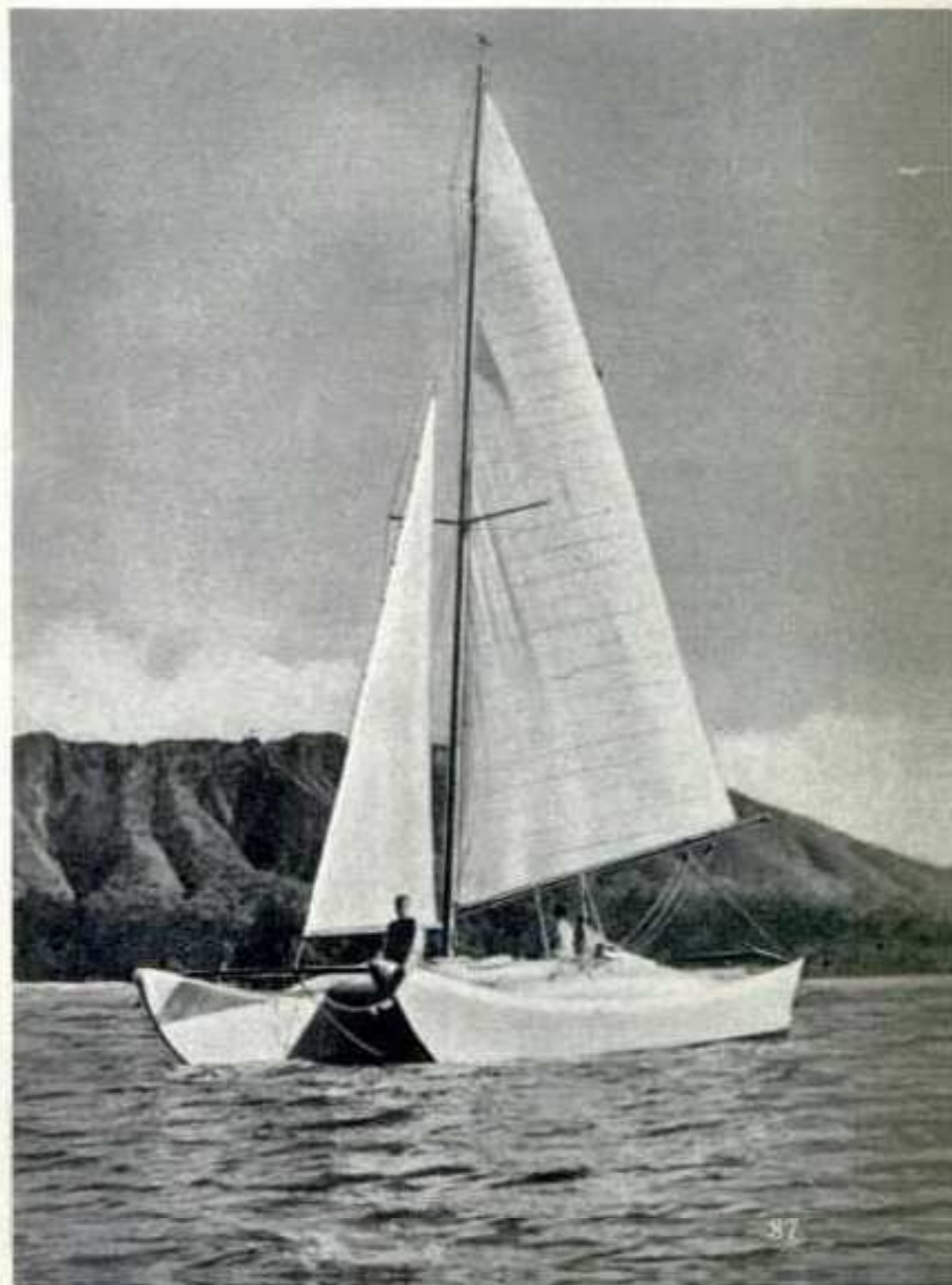
Six can be slept comfortably in the craft. Four are put in the wing section, which is entered by the hatches on deck, and there is space for one in each of the after hulls. Below, the Manu Kai carries only 370 square feet of sail, which is considerably less than half of that carried by one of the fastest catamarans developed in the early '30s.
